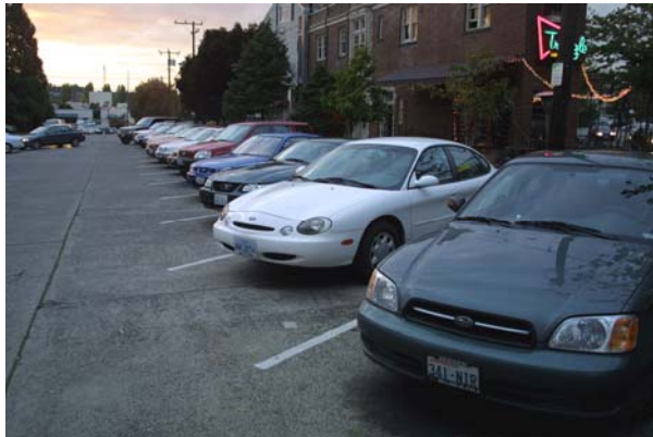
Back-in angled parking is safer and easier to manage than head-in angled and parallel parking. The most important safety advantage is the driver’s ability to see into the travel lane when pulling out of the parking stall.
