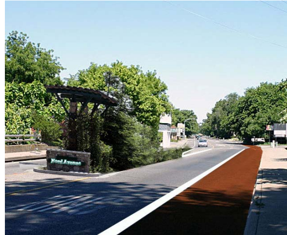
There is sufficient space on the bridge over Big Chico Creek to add a short median gateway treatment. Wider, colorized bicycle lanes can also help slow vehicles on the bridge and provide more buffer for pedestrians on the sidewalk.
