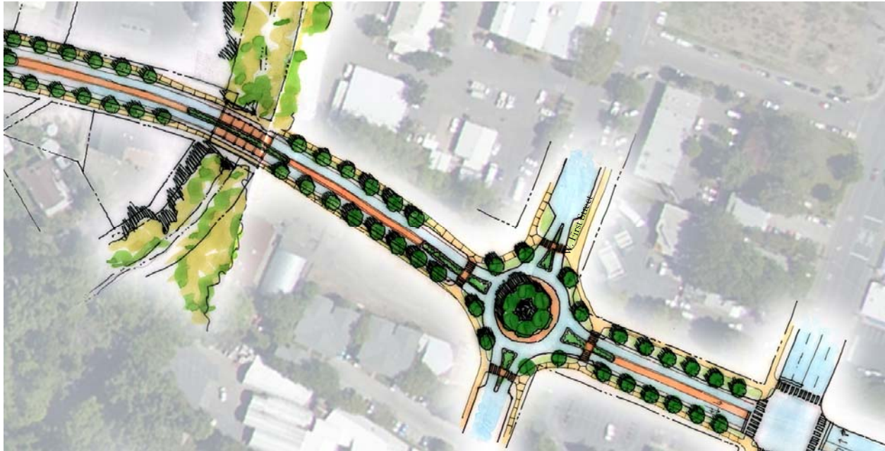
The transition from four-lane road to three-lane complete street could occur at the intersection of S.R. 32 and W. First Street with the introduction of a roundabout.
