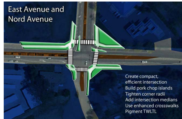
This diagram shows how as sidewalks and crosswalks are built special attention should be placed on providing curb extensions and crossing islands at large intersections so as to moderate speeds and help pedestrians cross the street.
